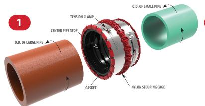
Lubricate large pipe end and gasket with soapy water solution. Loosen tension clamps to no more than five (5) serrations from strap end (see insert). Install the coupling over the large pipe end, just short of the center pipe stop. The center section of the nylon securing cage has to be unimpeded in order for centrical reduction to take place.
