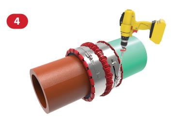
Lubricate smaller pipe end and gasket with soapy water solution. Insert pipe into coupling and take up slack with cordless drill or socket wrench. Complete installation by tightening tension clamp to 80 in/lbs. minimum torque at slow speed.
