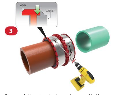
Ensure gasket is centered and properly engaged inside nylon securing cage (see insert) before tightening tension clamp. Tighten to 80 in/lbs. minimum torque at slow speed.
